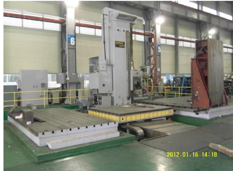
CNC Boring machine (D160 × 7000 × 2500 × 900)
