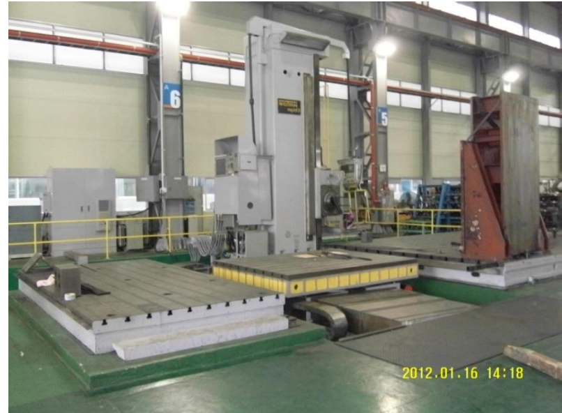
CNC Boring machine (D160 × 7000 × 2500 × 900)
