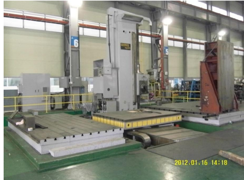
CNC Boring machine (D160 × 7000 × 2500 × 900)
